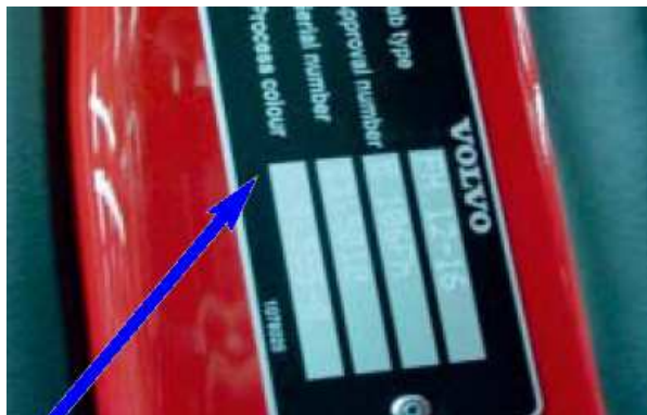
VIN PLATE FH + FM PAINTCODE LOCATION
